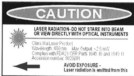
Avoid Exposure - Laser Radiation is emitted from this aperture.
